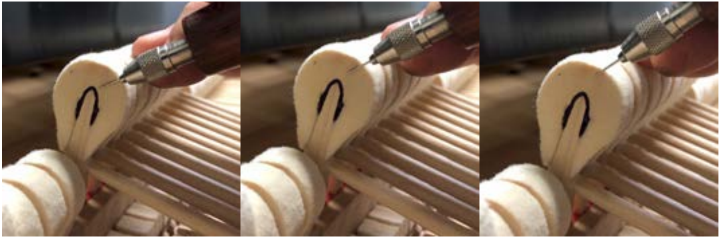
Suggested positions and depths of needle stabs in grand pianos.
