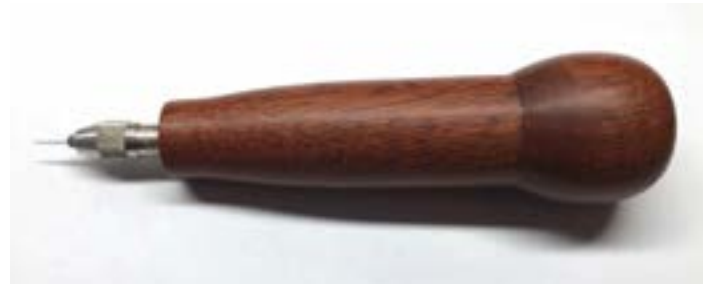
Single-needle voicing tool by Boaz Kirschenbaum, RPT.
