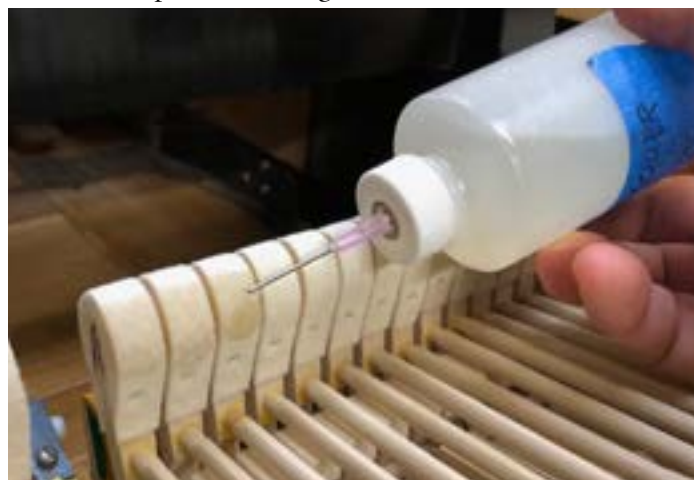
Increasing power and brightness by applying a lacquer solution to the shoulders.
