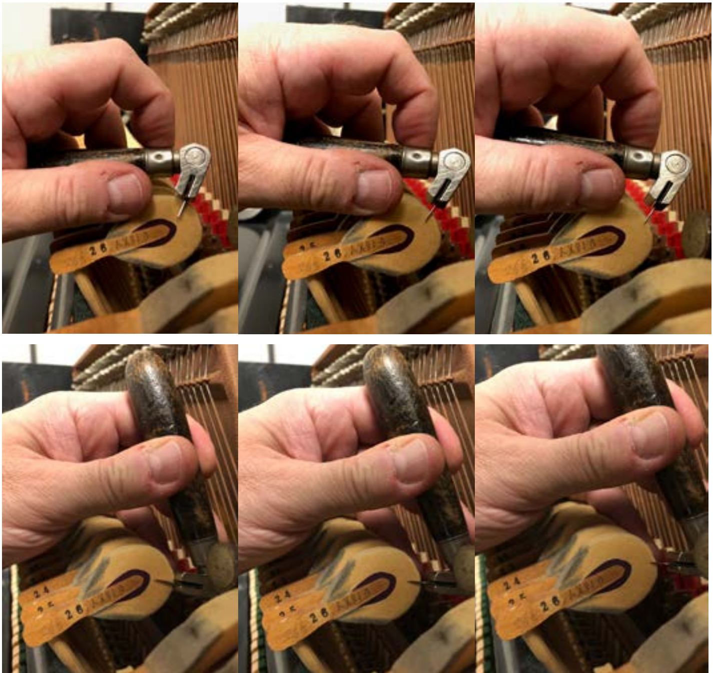
Suggested positions and depths of needle stabs in vertical pianos.
