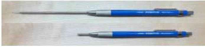
Retractable chopstick voicing tool.
