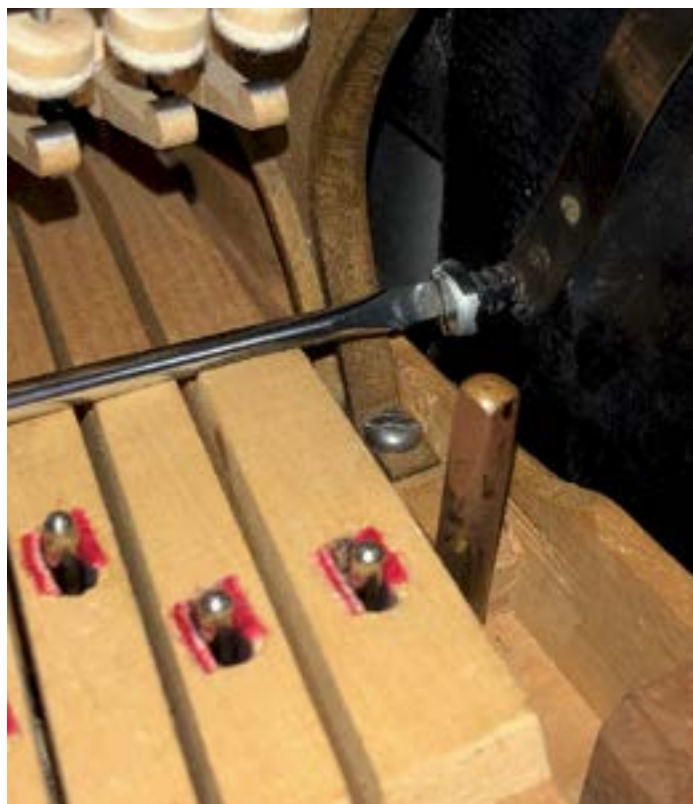
Adjusting the soft pedal shift stop screw.
