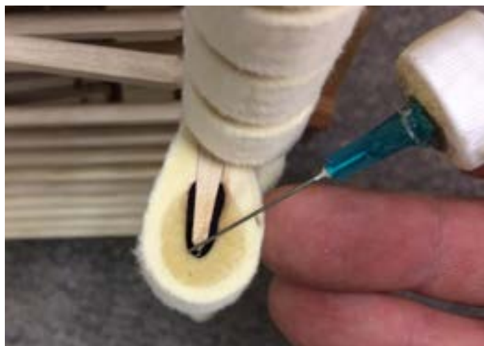
Increasing projection and volume in a hammer with softer felt.
