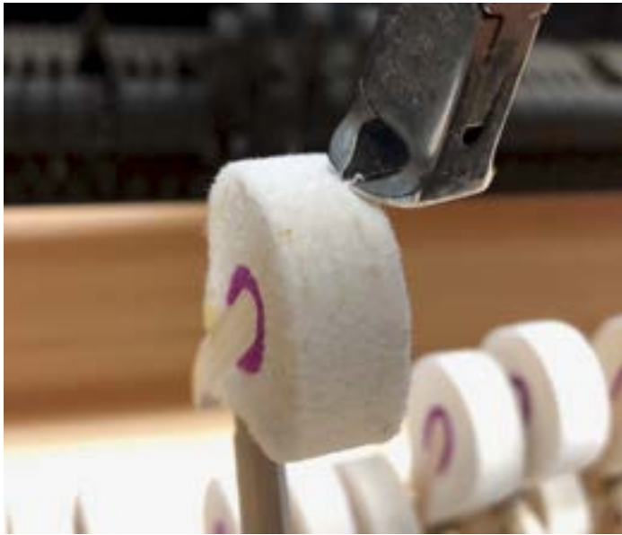
Extracting a broken needle from the hammer with center pin nippers.
