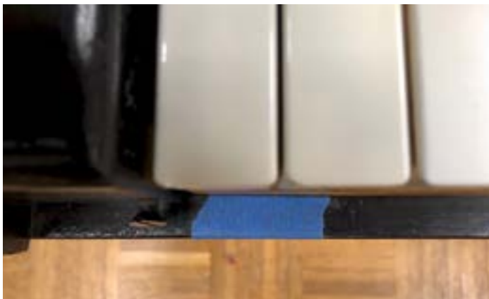
Front rail position marked on the keybed using painter's tape.
