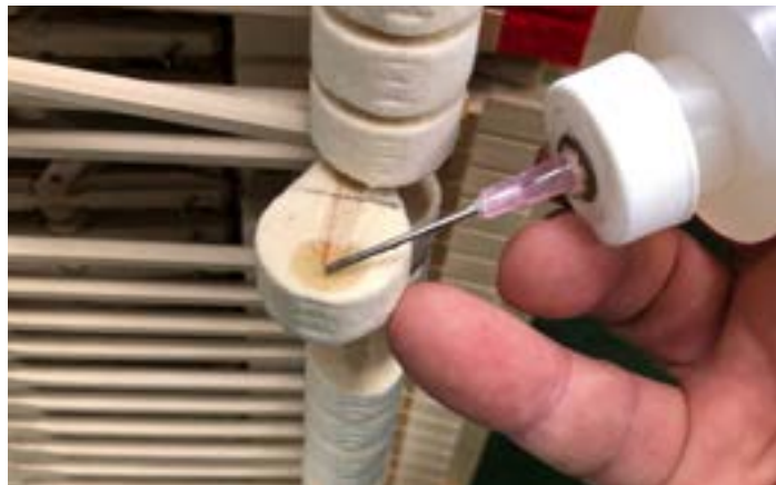
Increasing projection and volume in a hammer with dense felt.
