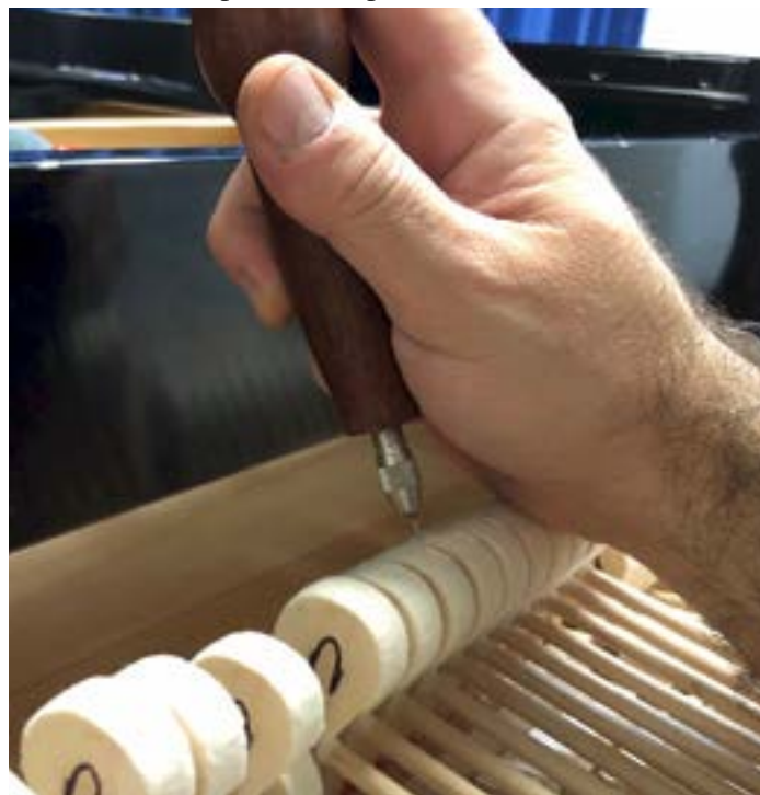
My technique for needling the aft (rear) shoulders.
