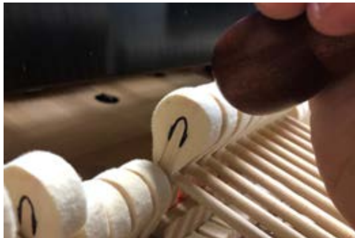
Resetting the felt by pounding it with the back of the voicing tool.
