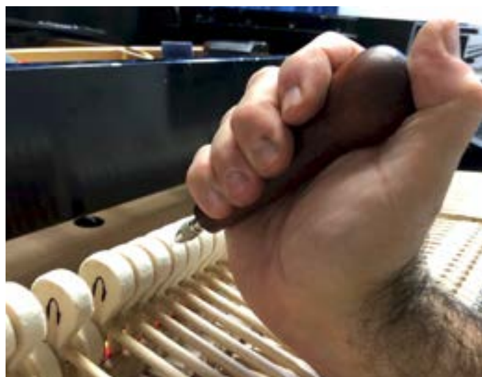
One position for needling fore shoulders.
