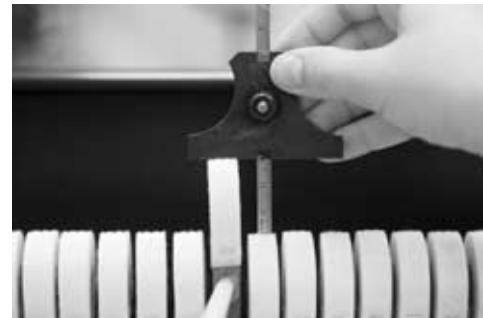
Figure 463 Measuring hammer travel at 6 mm key travel: The front of the action-leverage tester should be at the standard measurement position (13 mm in from the key front). The extra weight prevents the tool from rocking back a little on this piano. The depicted tester is made by Erwin's Piano Restoration.
