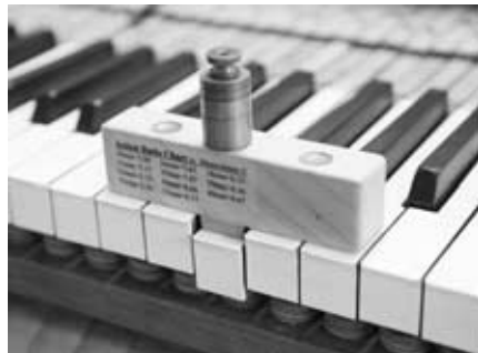
Figure 463 Measuring hammer travel at 6 mm key travel: The front of the action-leverage tester should be at the standard measurement position (13 mm in from the key front). The extra weight prevents the tool from rocking back a little on this piano. The depicted tester is made by Erwin's Piano Restoration.
