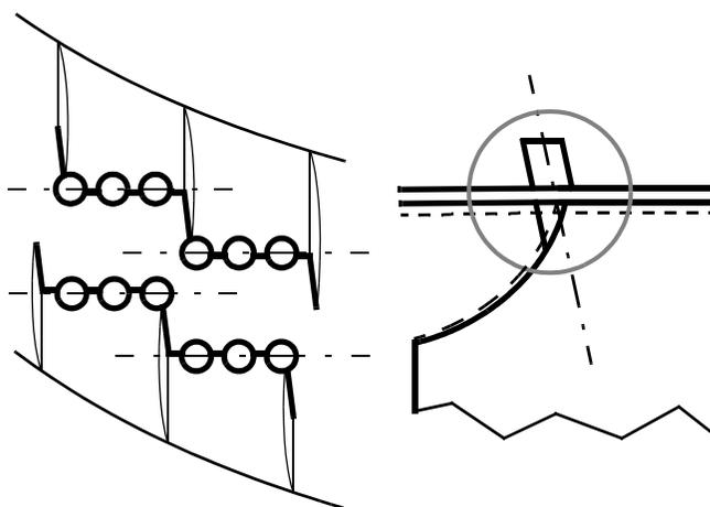
Figure 105 Bridge notches on a new bridge (cap) should start somewhat closer to the center of the bridge instead of at the exact center of the bridge pins. This compensates for the grooves that form in the bridge cap over time.
