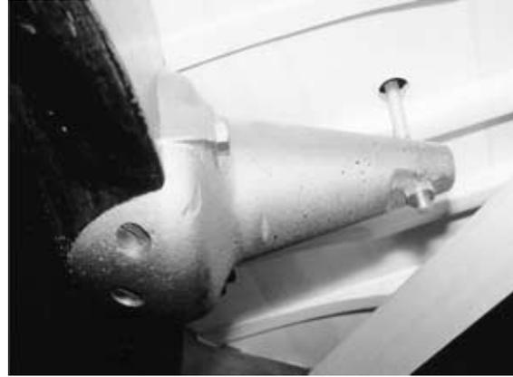
**Figure 33** The Steinway “bell” supports the plate and increases its rigidity in the treble (ca. 1985 Hamburg Steinway model C).
