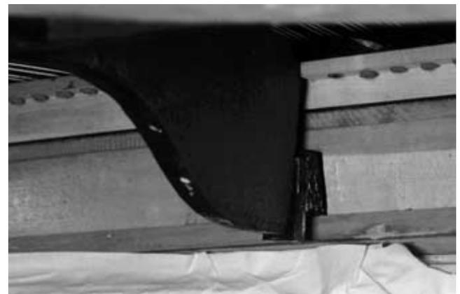
**Figure 36** The plate horn in modern Steinway & Sons grand plates is connected by a steel wedge to the metal shoe toe, which protrudes through the belly rail (see Figure 55 on page 29). The beams converge on the shoe behind the belly rail.
