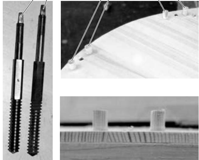
**Figure 32** Piano plate supports: nose bolts and rim dowels.
