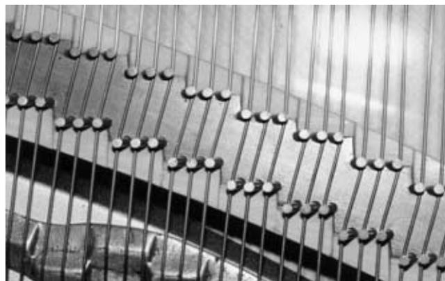
Figure 104 Notching of a replaced bridge cap.
