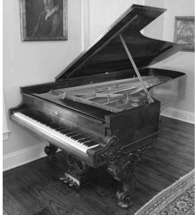
Figure 25 This 1878 Steinway 8'6" [259 cm] Style III concert grand is among the last “antique” Steinways with composite rim, open-face pinblock, and three-quarter plate. This model was made in parallel with the 8'9" [267 cm] “Centennial” concert grand, which had a full-size plate and was first made in 1875. Both were superseded by the composite-rim model D in 1878, and by the rescaled model D in 1884, which had a continuous, laminated rim and a full-size double cupola plate.
