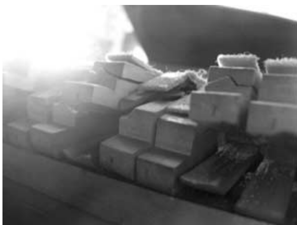
Figure 203 Damage to the backs of keys in an Érard vertical piano from ca. 1890, caused by corroded leads. Additional damage was caused by attempts to depress the keys, which had been immobilized by the expanded leads.
