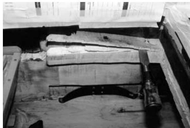
Figure 683 Chiseling out the treble end of the original pinblock. Chisel the top layer in one piece to facilitate duplicating the width of the pinblock.
