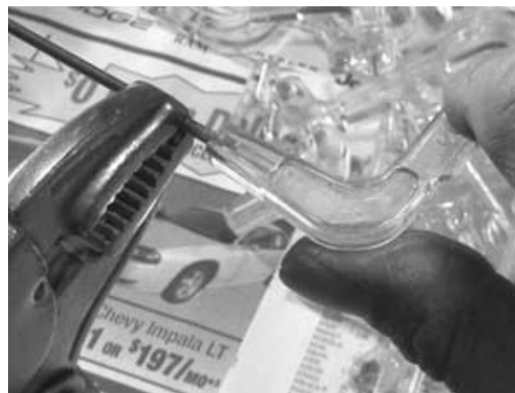
Figure 623 Winding a new elbow onto a sticker.
