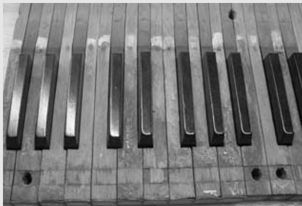
Figure 525 The person who removed ivories from these keys inadvertently pulled off wood strips from the front mortises. If the strips are not restored, the tops will click in those spots.
