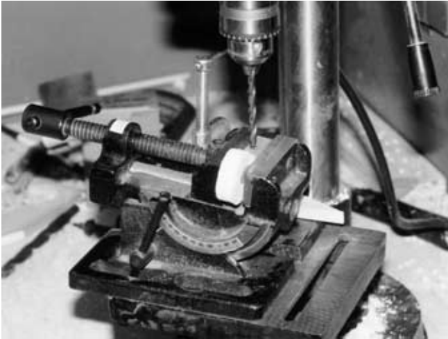
Figure 584 Angle vise set up on a drill-press table (shown with a bass hammer).
