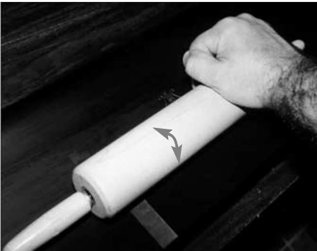
Figure 758 Pressing down the decal with a rolling pin.
