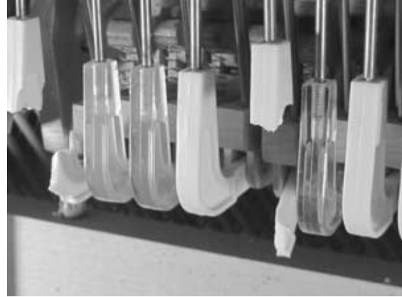
Figure 621 Broken plastic elbows.
