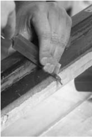
Figure 680 Cleaning the remaining wood from the stretcher with a chisel (a). Steaming the wood first (b) may reduce damage to the stretcher (courtesy Pianos Bolduc).
